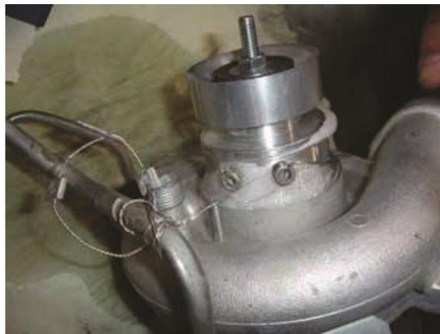
WRONG RESTRICTOR SEALING
